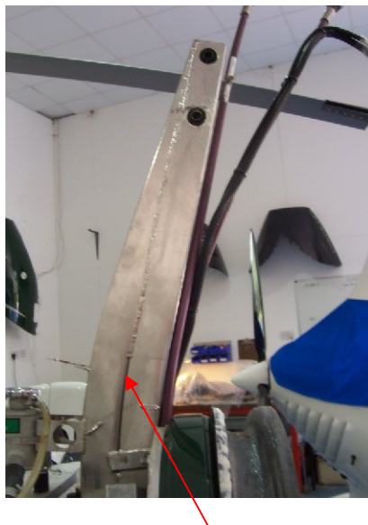
Extent of bend shown at top of mast
