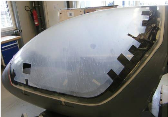
Canopy fixtured onto in-situ frame with foam & tape
