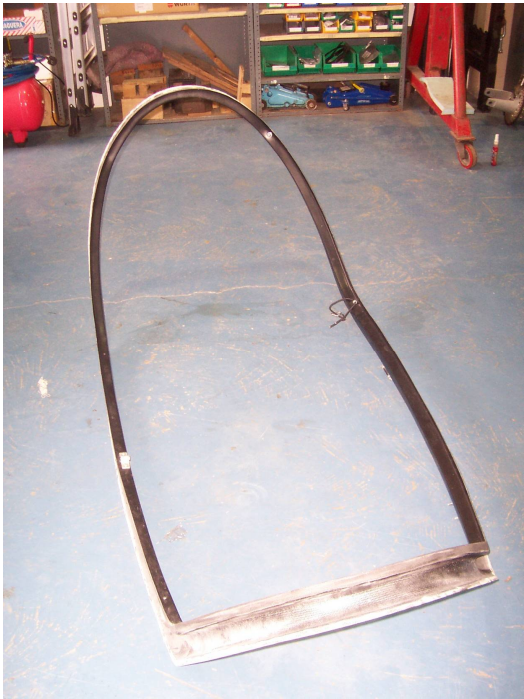
Canopy frame removed from aircraft
