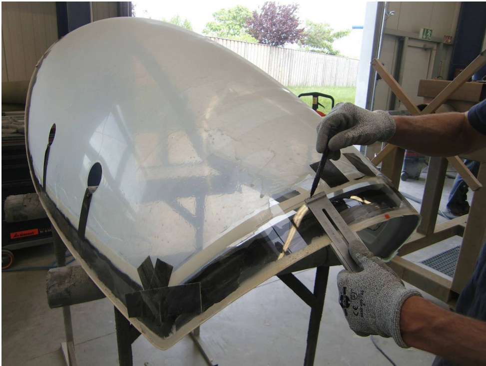
Marking-out for spray-painting
