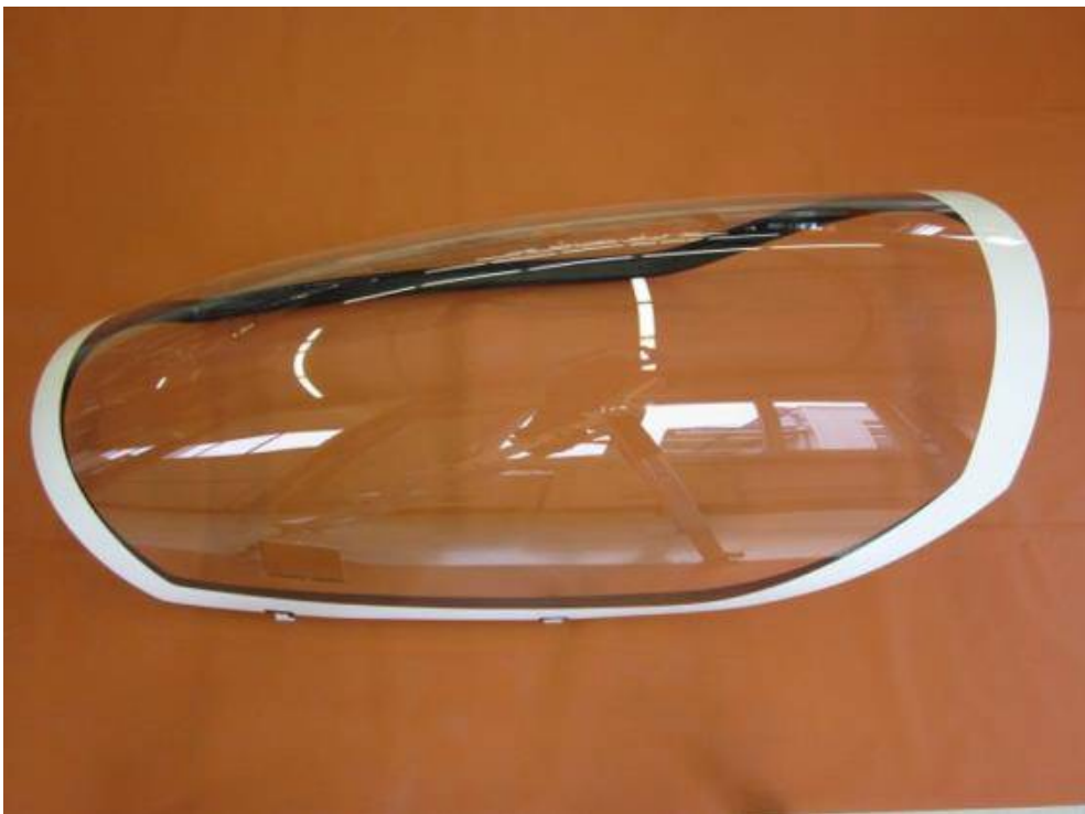
Canopy repair finished (without sun-shield)
