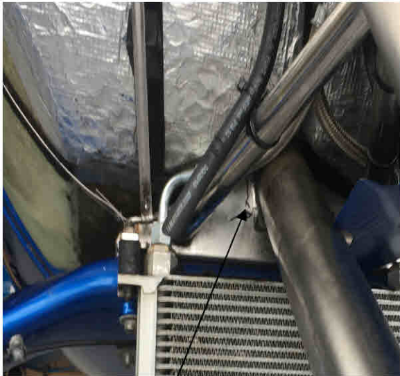
Crack position (could be either side of the mast)
