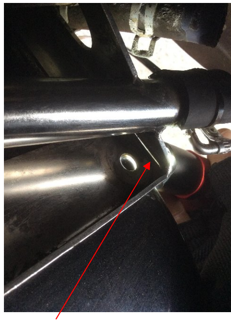
Crack position for this SRA-024 (mounting bolt removed and illuminated from rear)
