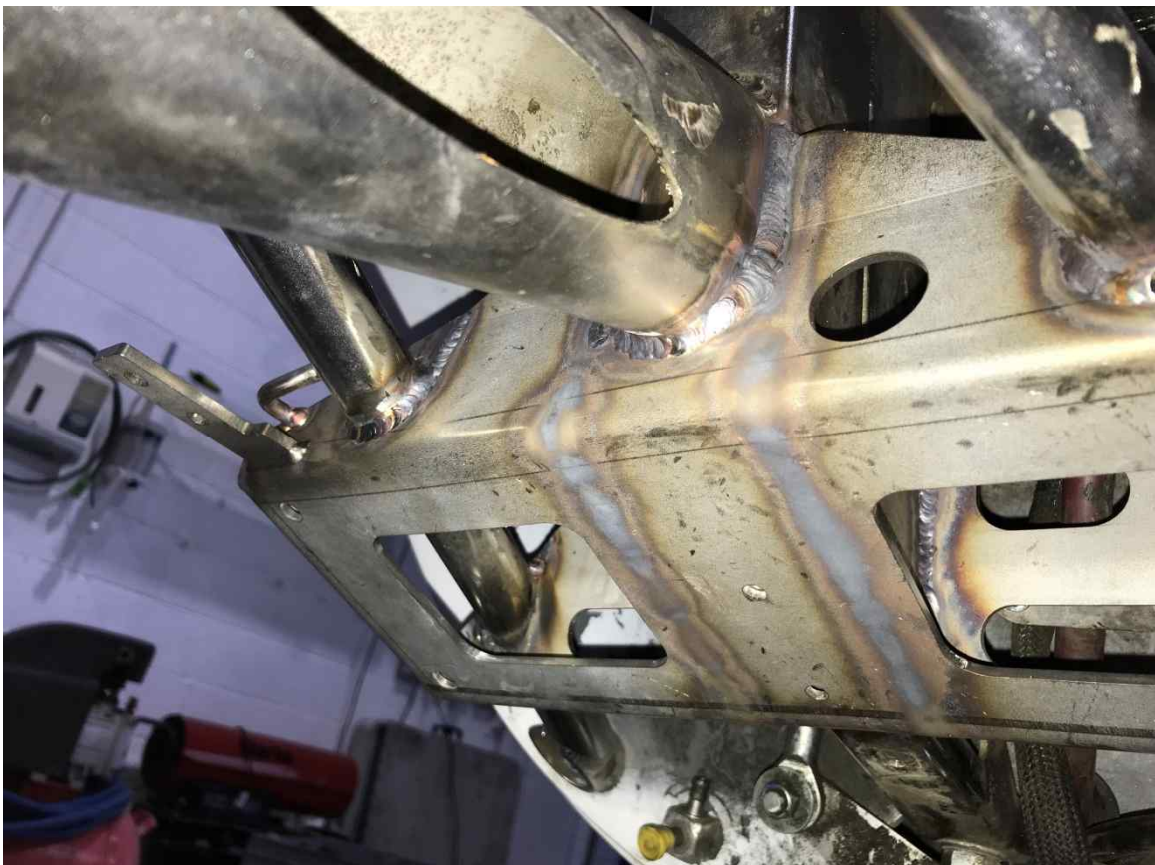
Underside view showing the weld to the keel tube.
