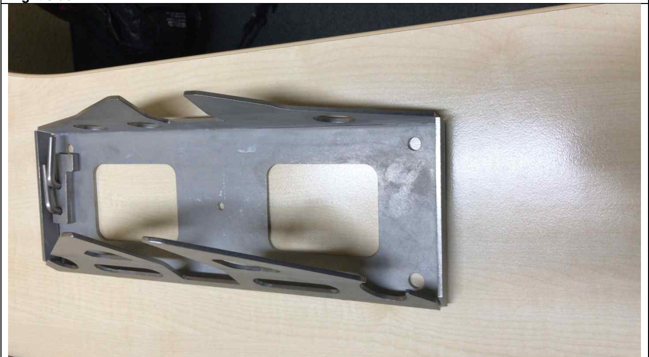
New bracket. Oil cooler mounting plate shown lying on top. The wireforms shown are not required. New bracket fitted, ready to clean up and weld
