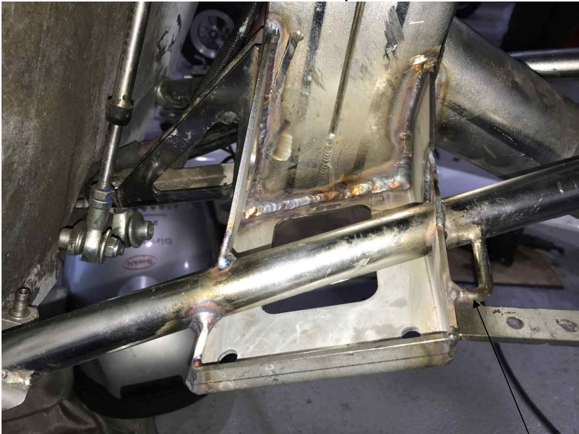
View of left bracket side. Note the original fuel tank strap bracket welded back into place
