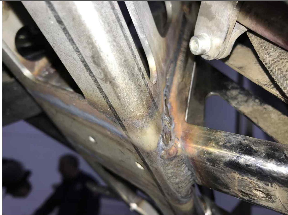
Underside view of the bracket weld to the front control stay
